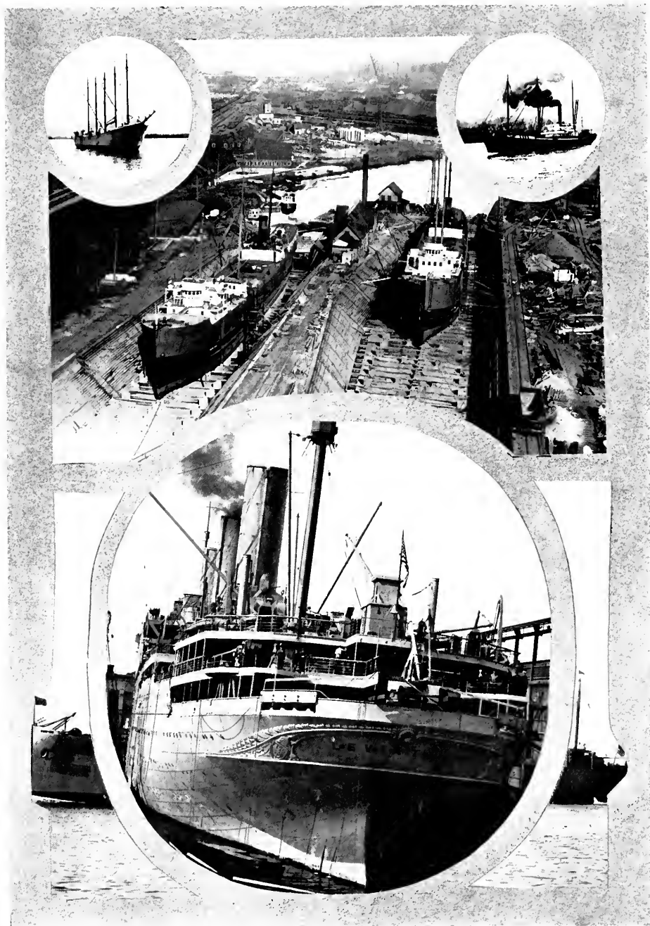
The upper picture is an interesting view of Great Lakes steamers in drydocks where they are being cut in two preparatory to passing through the Welland canal on their way to the ocean. The demand for steamers has led to a great many vessels too long for the canal locks to be treated in this manner. The lower picture is of the "Leviathan," formerly the "Waterland," which was seized by the Government and converted to military uses. Photos by the International Film Service.
